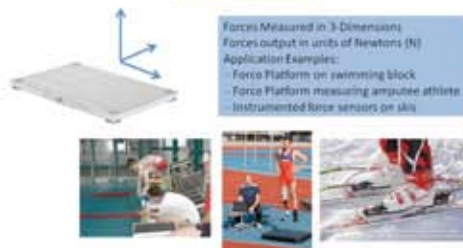
Figure 3: Examples of force measuring technologies that can be used to measure forces exerted by the athlete.
