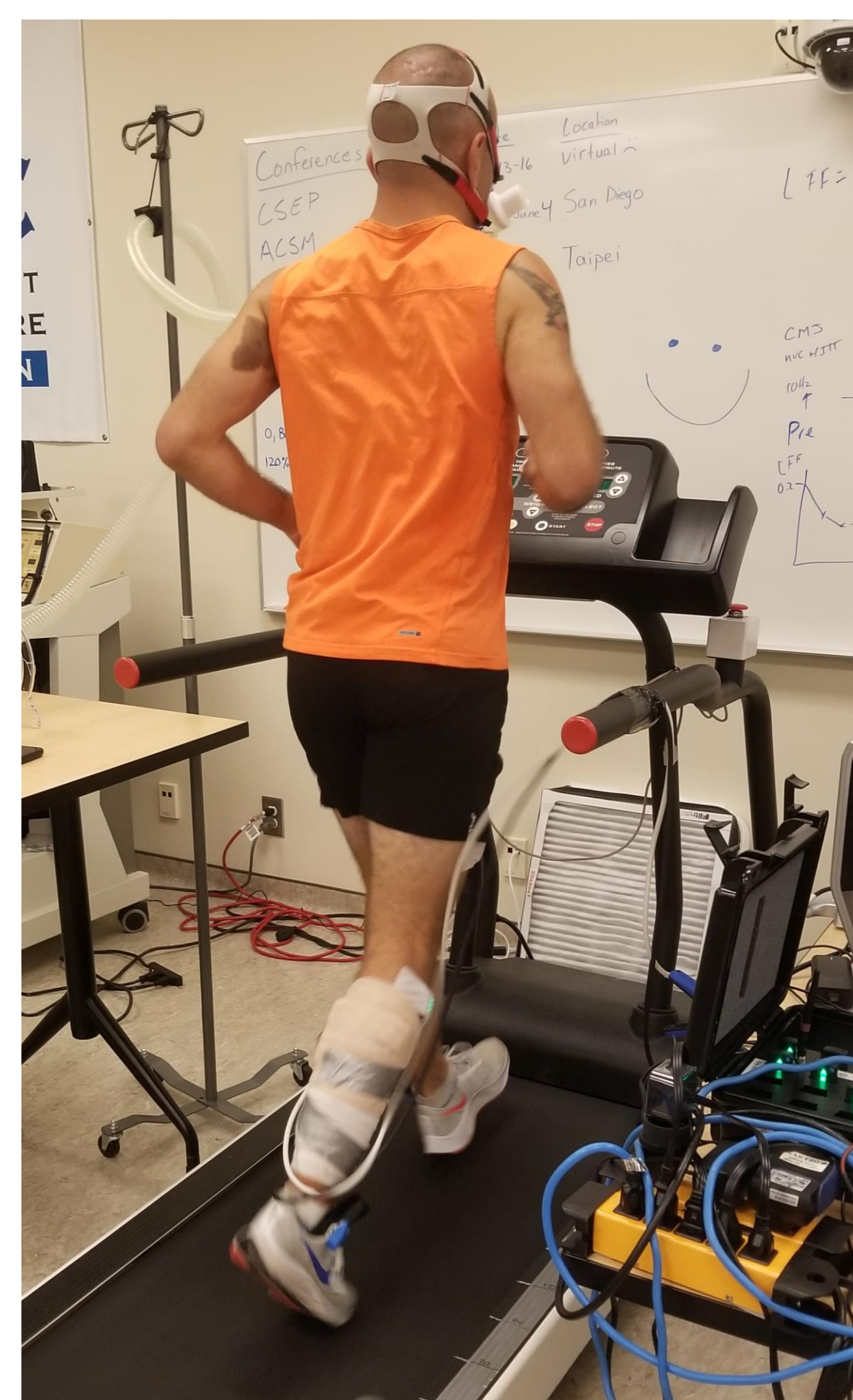
Figure 2. Experimental setup. Participants ran at 2.5 m/s while muscle and tendon length change was measured using ultrasound.
